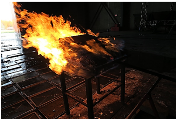
(c) Non-FRT Cedar Shake Roof / OSB Sheathing
